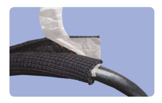
**FlexWrap® 3500** is a wrappable, damage-resistant sleeving designed to provide mechanical protection and acoustical noise suppression. Knit of monofilament and multifilament polyester yarns, the product offers a high level of component protection and is also very flexible.
